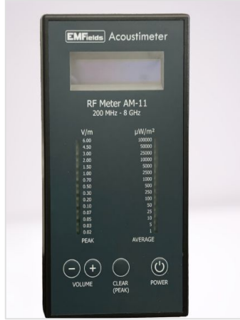
Radio Frequency (RF) Meter (Acoustimeter AM-11) (To measure the electromagnetic waves)
